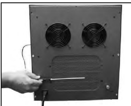
Inlet Air – Condenser (Back) Side•
