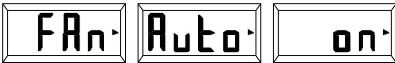
The panel will show the word "fan" for a few seconds and then change automatically to the current fan setting, either "auto" or "on". To change the
