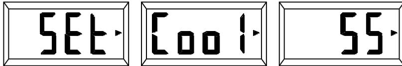
To change to your desired wine cellar temperature press either of the panel buttons until the desired temperature is shown. If the desired temperature is the
