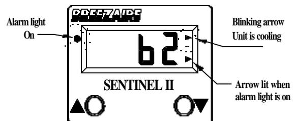
When the cooling unit is plugged in and receiving electrical power the top arrow will be lit. This top arrow will blink when the compressor is operating and the unit is cooling. The middle arrow is lit when the programming is being changed. The bottom arrow is lit when the cellar's temperature exceeds the alarm set temperature. Also at this point the red alarm light will be on.
