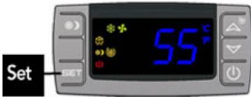
The cooling unit is factory preset with a Minimum Set Point of 58°F and a Temperature Differential of 4°F. This means that the cooling unit will turn on when the display rises above 62°F (58°F + 4°F), and turn off when the display falls below 58°F. In this example, the average temperature inside the cabinet will be 60°F.
