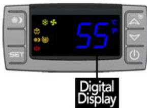
The temperature displayed on the control indicates the real-time air temperature as measured by Probe 1 (P1) located on the inlet grill of the cooling fan.
