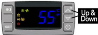
To view the “Low Temp” recorded by the cooling unit, press the “Down” button once
