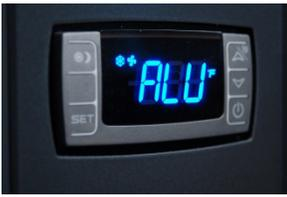
**HIGH TEMPERATURE ALARM:** The factory preset for this setting is “70”.
