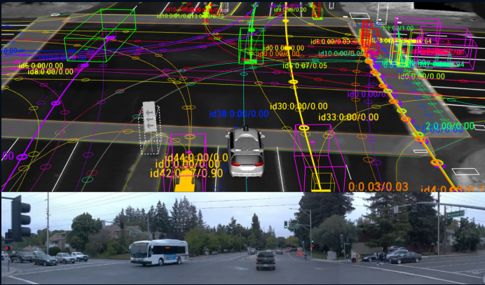
↑ The simulated imagery shown demonstrates how Waymo's software assigns predictions to each object surrounding our vehicle—other vehicles, cyclists, pedestrians, and more.
