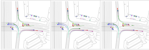
Figure 3 | MPS creates diverse (multi-modal) rollouts.
