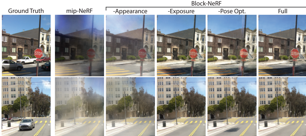
Figure 7. Model ablation results on multi segment data. Appearance embeddings help the network avoid adding cloudy geometry to explain away changes in the environment like weather and lighting. Removing exposure slightly decreases the accuracy. The pose optimization helps sharpen the results and removes ghosting from repeated objects, as observed with the telephone pole in the first row.
