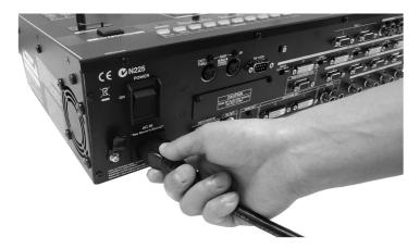
2. Secure the power cord in place with the cord hook.
