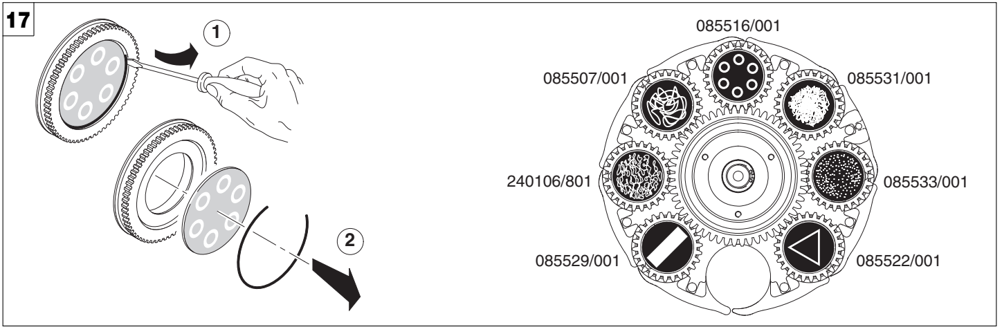
Replacing rotating gobos ( \varnothing 25.7 mm - max 23 mm image – thickness max 1.1 mm) - Fig. 17
