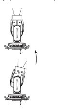
Operation with option Invert Tilt  $\,\,^{\diamond}$  On (Pan conventionally represented at 0% and option Invert Pan  $\,\,^{\diamond}$  Off)
