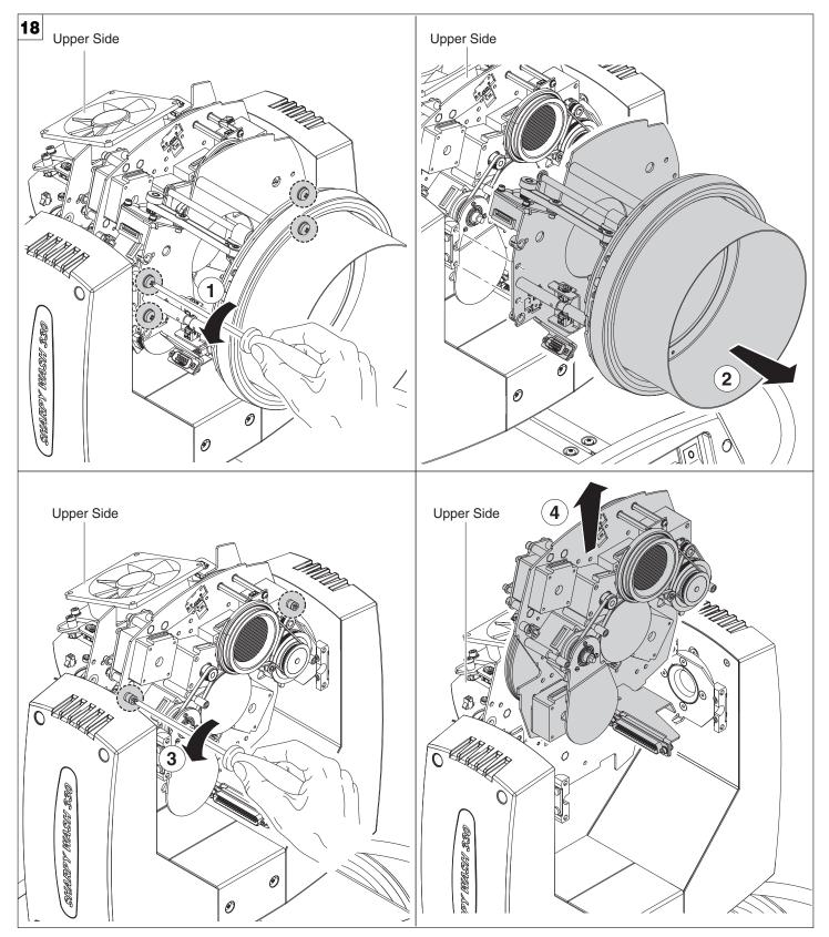
Extraction of the effect modules - Fig. 18 IMPORTANT: Grasp the modules using the support structure and not the details which could get damaged. Insertion of the effect modules: Repeat the operations indicated in Fig. 17 and 18 in reverse order.
