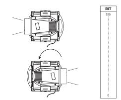
Operation with option InvertPan  $\,\,\hat{\circ}\,\,$  On (Tilt conventionally represented at 14% and option Invert Tilt  $\,\,\hat{\circ}\,\,$  Off)
