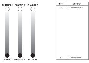
**IMPORTANT:** The lamp dim to half power 1 second after all the 3 channels stay at 0% level. The lamp goes back to full power when the channels level is put higher than 0%.
