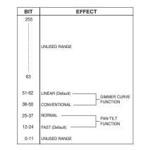
The functions are actived passing through the unused range and staying 5 seconds in necessary level.
