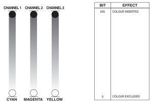
**IMPORTANT:** The lamp dim to half power 1 second after all the 3 channels stay at 100% level. The lamp goes back to full power when the channels level is put lower than 100%.
