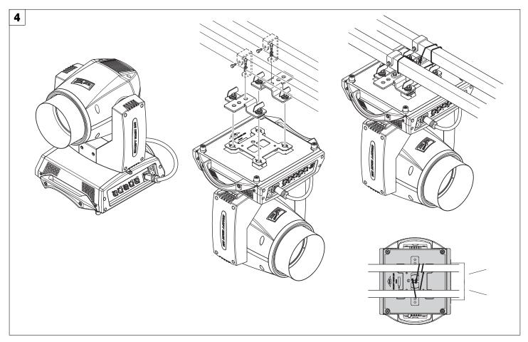
**Installing the projector** - Fig. 4 The projector can be installed on the floor resting on special rubber feet, on a truss or on the ceiling or wall.
