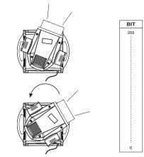
Operation with option InvertPan  $\circ$  On (Tilt conventionally represented at 14% and option Invert Tilt  $\circ$  Off)
