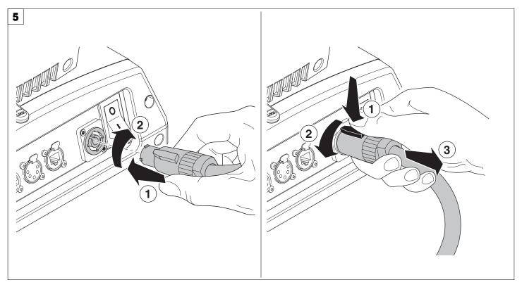
Connecting and disconnecting power cable - Fig. 5
