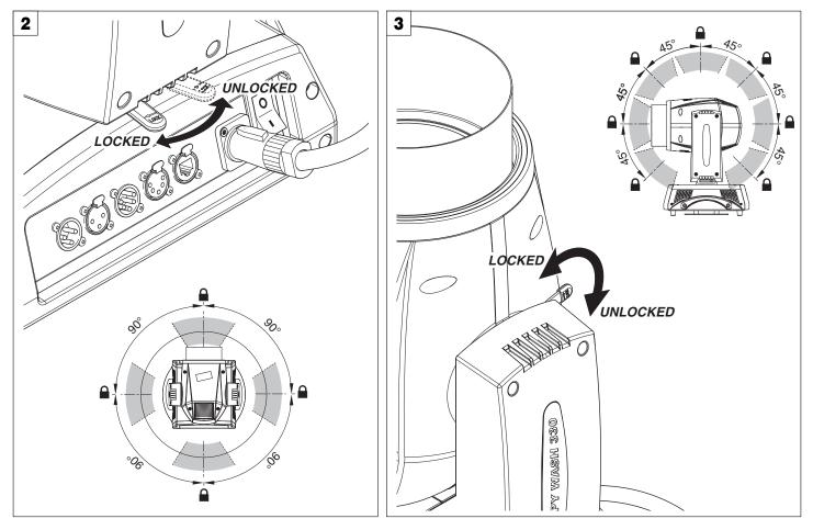
PAN Mechanism Lock and Release (every 90°) - Fig. 2
