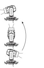
Operation with option Invert Tilt  $\degree$  On (Pan conventionally represented at 0% and option Invert Pan  $\degree$  Off)
