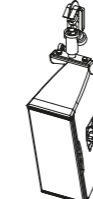
T10 point source or Ti10P with Z5371 T Flying bracket Z5010 TV spigot with fixing plate Z5012 Pipe clamp for TV spigot
