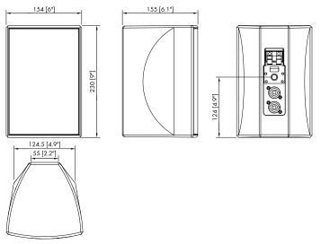
Fig. 12: E5 cabinet dimensions in mm [inch]
