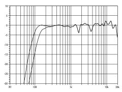
Fig. 11: E5 frequency response, standard and CUT modes
