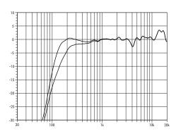
Fig. 9: E4 frequency response, standard and CUT modes.
