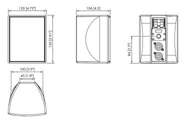
Fig. 10: E4 cabinet dimensions in mm [inch]
