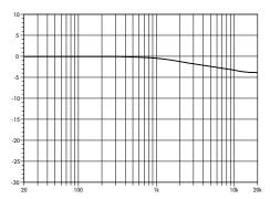
Fig. 3: Frequency response correction of HFA circuit
