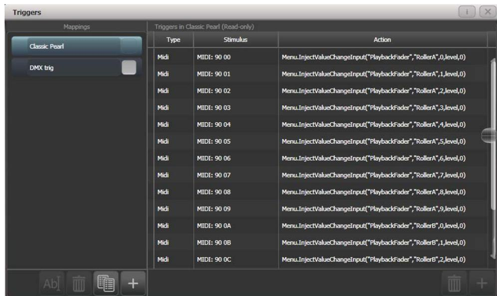
To delete a trigger from the mapping, select it in the list and press the rubbish bin button at the bottom.
