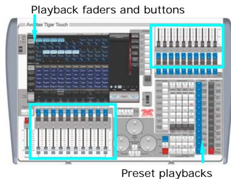
The Tiger Touch has 600 playbacks, in 60 pages of 10. In addition, you can store 10 'preset' playbacks on the faders at the top right of the console. These also have multiple pages, selected using two of the macro/executor buttons below.
