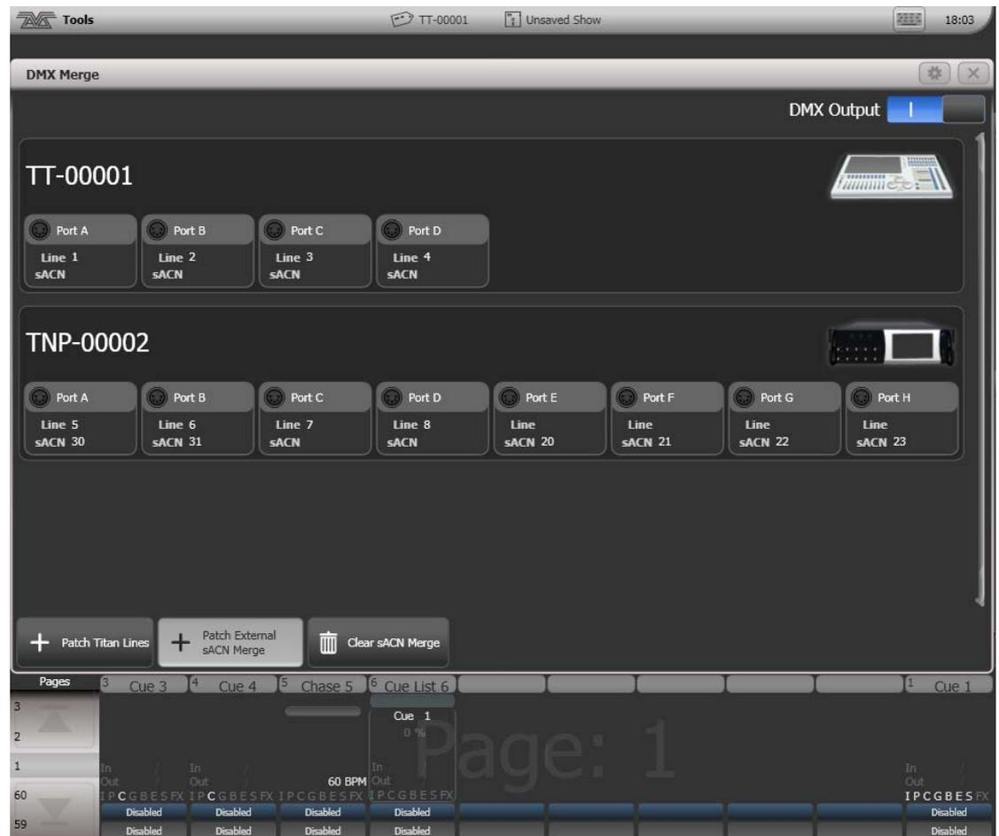
To configure an output port, click on Patch Titan Lines, enter universe number then click on a port to assign.
