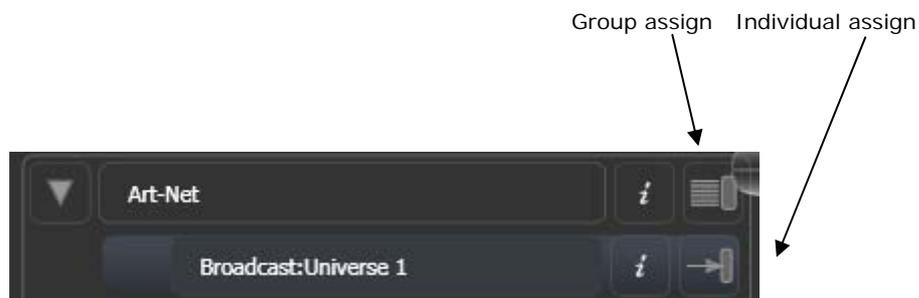
To assign a node to a line, click on the arrow on the node (the node will be highlighted), then click the line you want to assign to it.
