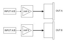
D12 Input/Output routing "Dual Channel"
