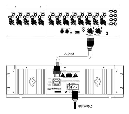
The **ML3000** console range is supplied with the **RPS11** power supply unit. A redundant (backup) **RPS11** may be connected using the second DC input socket. For early models, use the optional **RPSD2** combiner unit to connect a backup supply.
