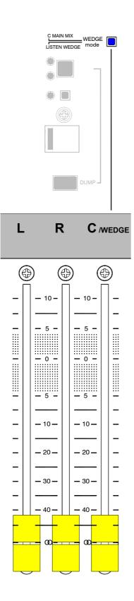
**WEDGE MODE**. This underpanel mode switch configures the C output to become the engineers monitor when the console is used for the stage monitor application. When pressed the monitor source is routed in mono through the C insert and fader to the main output. The C mix bypasses this section and is available from the matrix outputs if needed. The switch is protected to prevent accidental operation. Use a pen or pointed implement to select the required mode.
