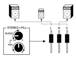
**LCR PA.** LCR systems are increasingly popular in large installed or touring systems. They comprise three main speaker stacks, left, centre and right to provide better coverage of a large audience. In some situations C is used only for sounds such as vocals to lift them out of the mix making them more intelligible, leaving backing instruments in the LR speakers. In other situations individual sounds are panned between the speakers according to source position.
