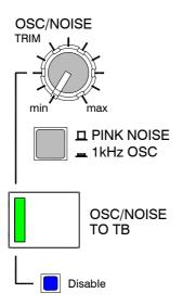
WARNING: The generator is capable of producing a high level continuous signal. To avoid damage to the speakers check that the generator and output levels are turned down before you route the test signal to the outputs. **OSC/NOISE TRIM**. Adjusts the level of the oscillator or noise signal from -30 to +10dB.
