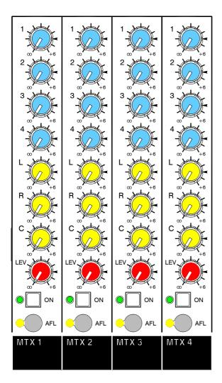
**MIX CONTROLS** Each of the 4 groups, L, R and C can be mixed into the matrix. The source is derived post-fader. Adjust the level clockwise from fully off to +6dB boost. The '0dB' position is marked.
