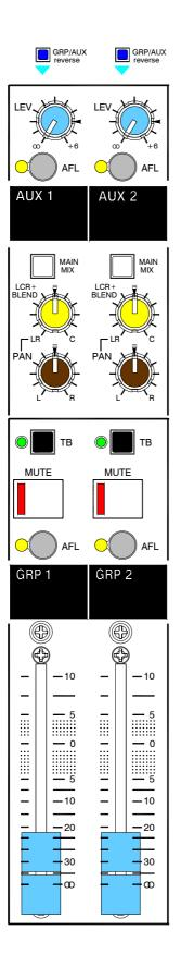
**GRP/AUX REVERSE MODE** This switch reverses the group fader and aux rotary master sections. It is underpanel to protect it from accidental operation. Use a pen or pointed implement to select the required setting. The default up position is flush with the panel.
