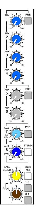
These controls send the channel signal to the audio groups 1-4 and aux sends 1-8. The layout is the same for both the mono and stereo channels. For the stereo channels the left and right signals are combined to feed the mono auxes.
