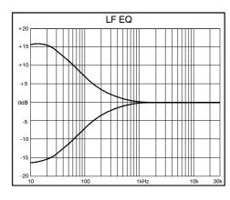
**EQUALISER**. The channel equaliser provides adjustment of 4 independent frequency bands. Each has cut/boost and the mids have frequency sweep controls. HF and LF are shelving. HM and LM are peak/dip to affect the chosen band of frequencies.
