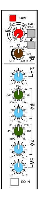
**+48V**. Switches +48VDC to the channel input XLR for powering microphones or DI boxes that need phantom power. The power is current limited through 6800 ohm resistors to pins 2 and 3.
