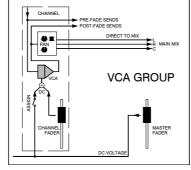
VCA groups affect the channel post-fade sends. They do not affect the pre-fade sends. Use VCA groups for level control. Use audio groups when you need to insert signal processing or feed the matrix.
