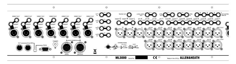
**CHANNEL INPUT** XLR input for mic or line level signals. Pin 2 hot. Phantom power is fed to pins 2 and 3 through 6k8 series resistors when the front panel +48V switch is pressed.
