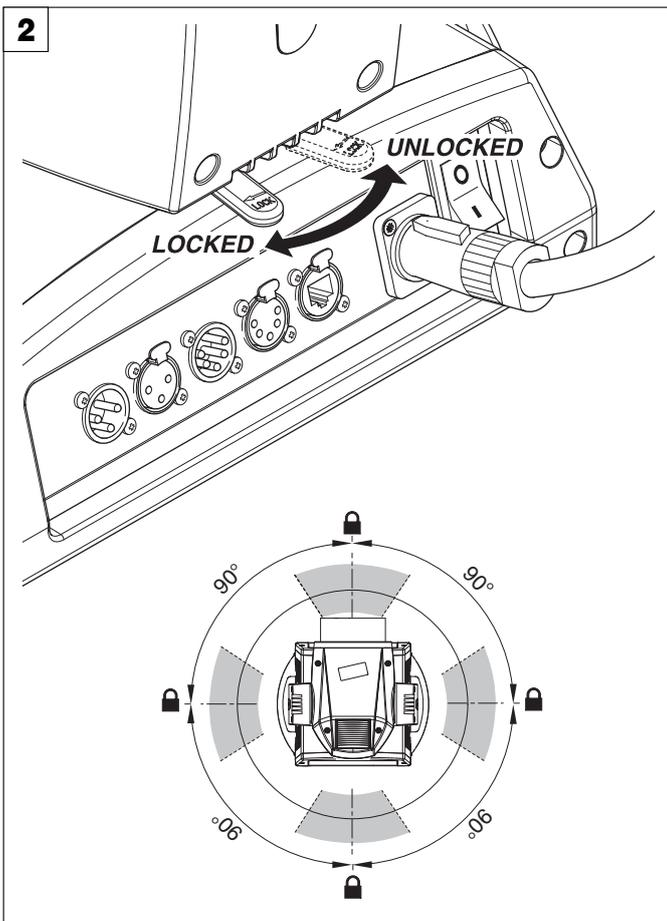
PAN Mechanism Lock and Release (every 90°) - Fig. 2
