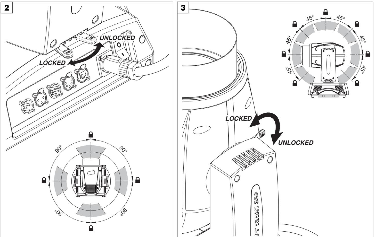
TILT Mechanism Lock and Release (every 45°) - Fig. 3
