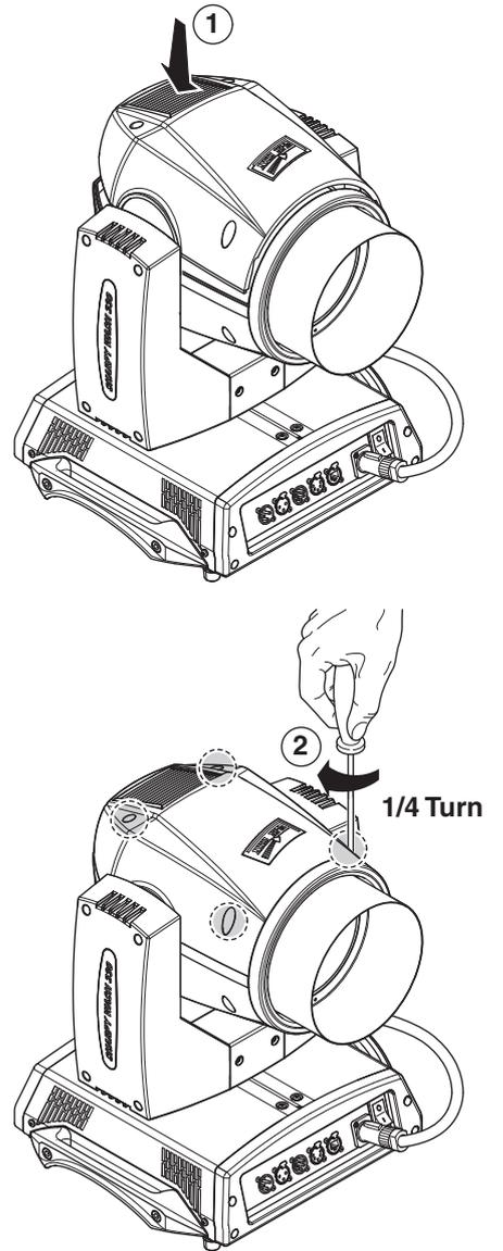
Locking and releasing Pan and Tilt movements - Refer to the instructions in the UNPACKING AND PREPARATION section.
