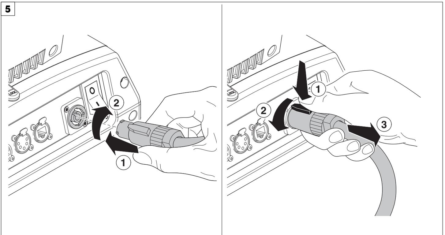
Connecting and disconnecting power cable - Fig. 5
