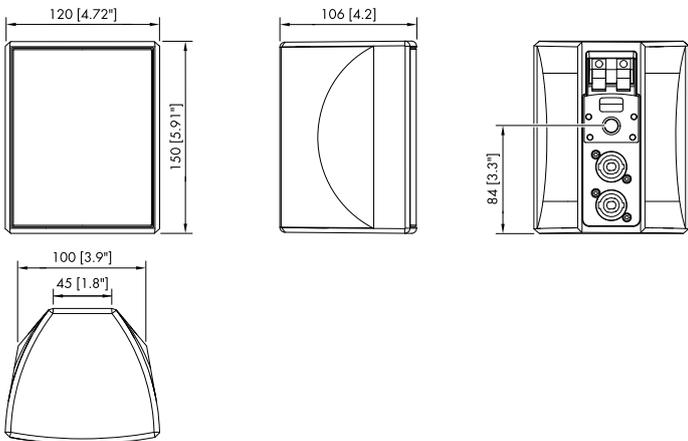
**Fig. 10: E4 cabinet dimensions in mm [inch]**
