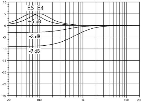
**Fig. 4: Frequency response correction of the CPL circuit**
