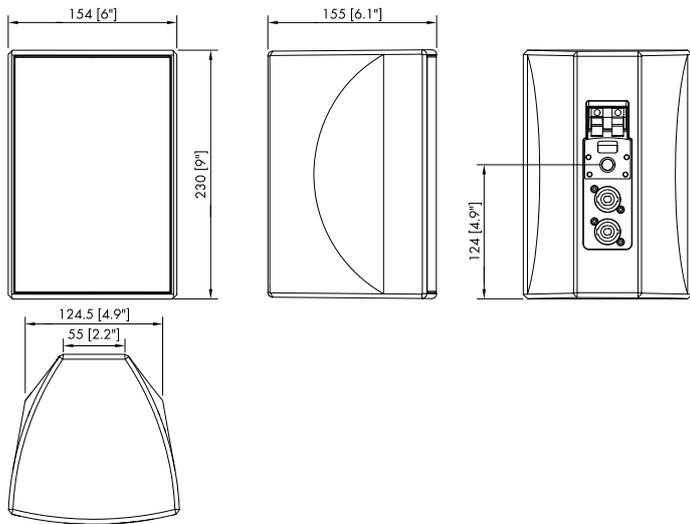
**Fig. 12: E5 cabinet dimensions in mm [inch]**
