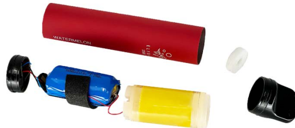
Fig. 1: usually a disposable ENDS is composed by 1- airflow activator, 2- battery, 3- casing, 4- plastic tube containing cotton imbibed with e-liquid.
