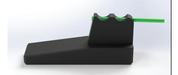
3. Trim fiber optic rod to just beyond the muzzle end of the front sight, leaving around .050" exposed.
