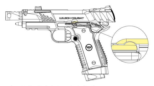
3. Retract the slide to align the take down notch of the slide with the inner lug of the slide stop, completely push the slide stop out and remove.
