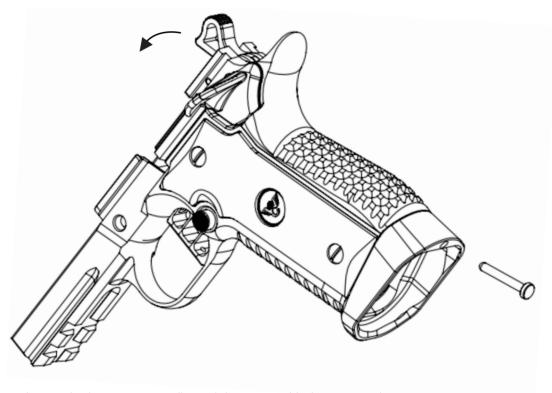
8. Lower the hammer carefully, so it is at rest with the front of the hammer slot in the frame. Failure to do so can damage your firearm.
