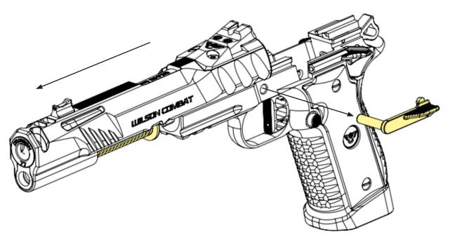
4. Slide the assembly forward to remove from the frame, while capturing the recoil spring and guide with your fingers cupped.
