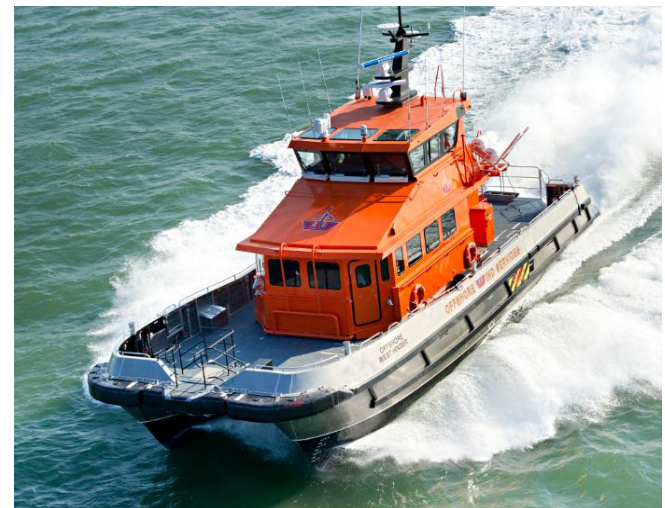
Offshore West Hinder, 21m SouthCat crew transfer vessel built 2012 for Offshore Wind Services
