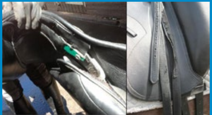
To the left, a front view of a saddle in which the left panel is displaced, because of a missing adjustable gullet screw, exposing the tree. To the right, a potentially dangerously worn stirrup leather.
