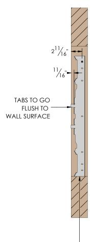
**BOTTOM OF BRACKETS** ALIGNED WITH BOTTOM OF WALL OPENING-
