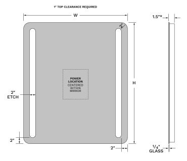
\* Total depth is 1.5" for marine-grade housing and 2" for traditional steel housing.
