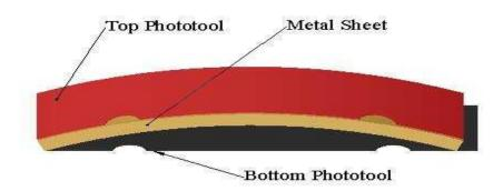
The film registration is achieved at the phototool production stage. Providing any curvature is removed during the printing operation, registration is not an issue. This curvature is removed by either mechanical pressure (by sandwiching the metal and films between 2 sheets of glass) or by vacuum. (A flexible top sheet pulling down on a rigid glass lower sheet.
