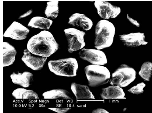
Figure 2.9: Photograph of the 3-D bed material captured by an electronic microscope.
