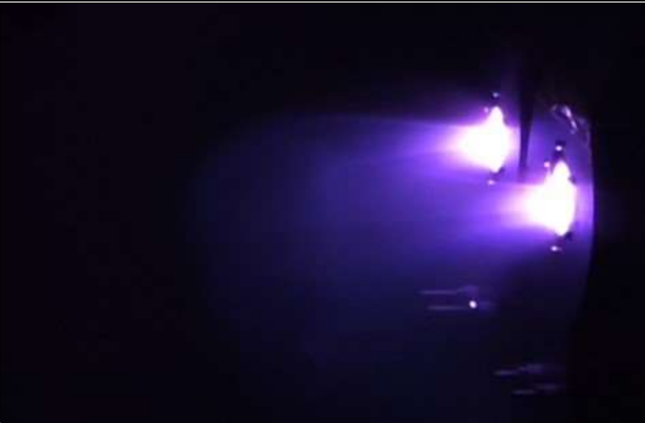
Cluster in operation with "MF ARCH" configuration.
