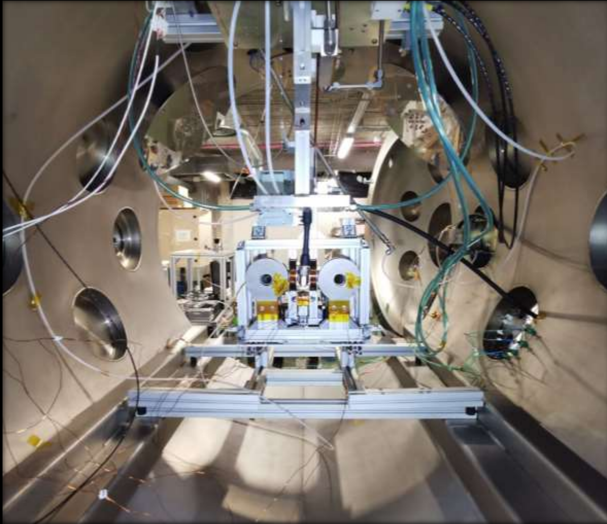
Cluster thruster installed in the EP2 group vacuum chamber
