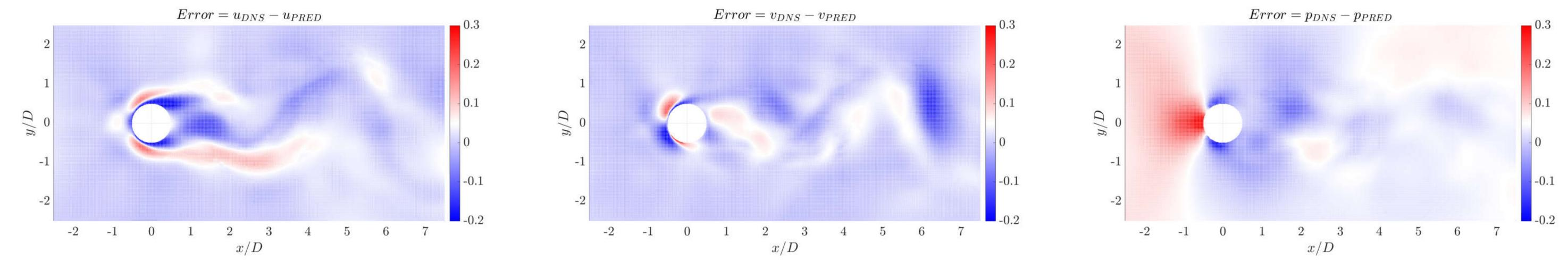
Synthetic data from Direct Numerical Simulation are used as a reference for error calculation
