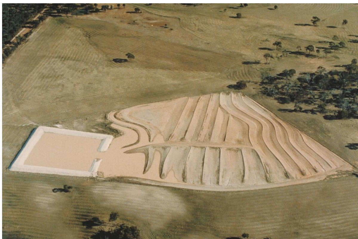
Figure 1. An example of a roaded catchment (source Department of Primary Industries and Regional Development (DPIRD)).
