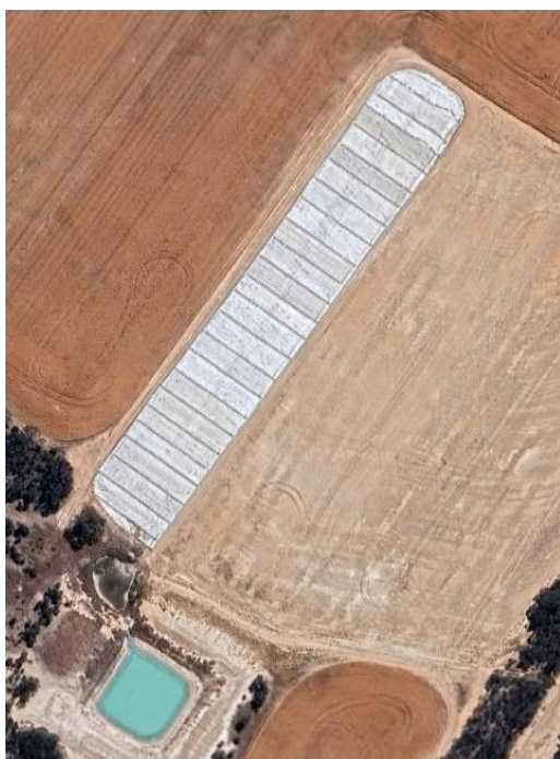
Figure 8. Satellite image of Wandel site PVC tarped catchment system, 2025
