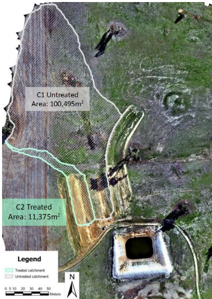
Figure 6. Satellite image of the Goss dual catchment system, with the Digital Elevation Model (DEM) outlining calculated catchment size, C1 untreated (brown) and C2 treated (Green).
