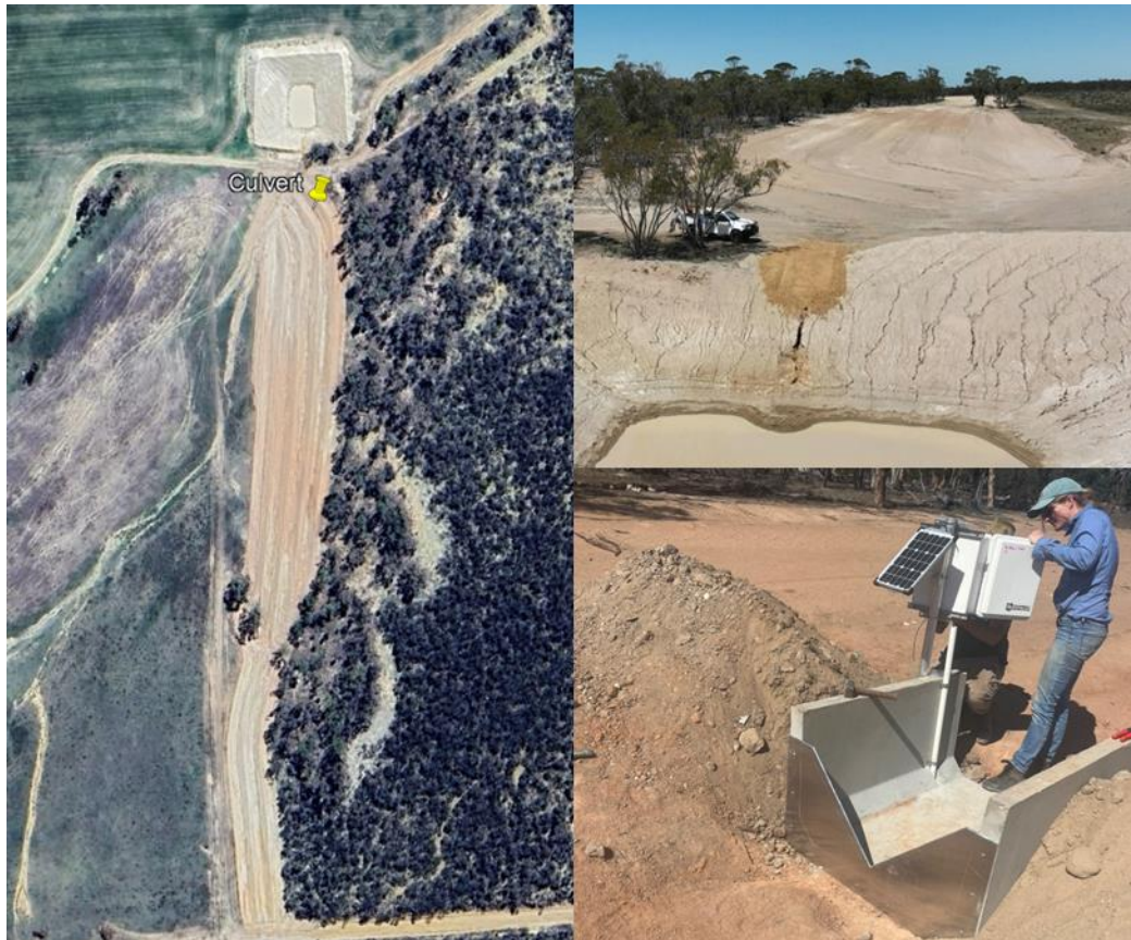
Figure 5. Satellite image of Giles roaded catchment, culvert and dam system, 2025(left). Drone image looking up the roaded catchment (right-top) and the V-notch weir and logger box (right-bottom).
