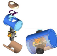
Figure 13. BESST in ScanEagle payload bay
