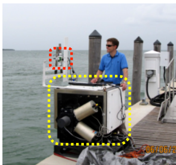
Figure 10. BESST (top-red) and M-AERI (bottom-yellow) mounted on pier
