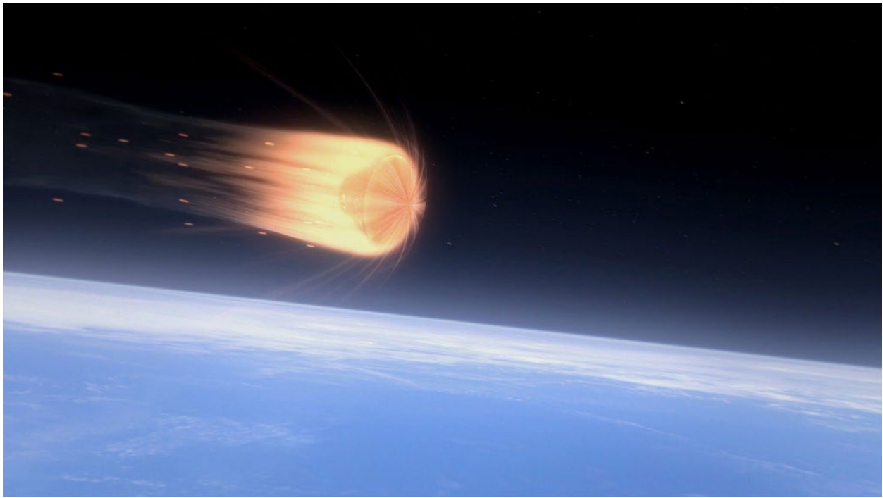
Figure 31: Orion with its base heat shield facing Earth as it encounters the first areas of the discernable atmosphere around the planet and the temperature around the spacecraft begins to build up (Siceloff).
