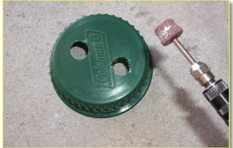
You will need to find a brake fluid supply bottle which will hold the extra brake fluid to be pumped to the brake reservoir when it is bled out, You can find it at Walmart at their "Camping equipment" section. The bottle has to be strong and have a tight seal and will hold at least 20 psi of pressure. Two holes need to be drilled to accommodate the connectors one which will be connected to the air source, the other to the custom made reservoir cap. Besides drilling out the hole I also used the Dremel to smooth out the edges.
