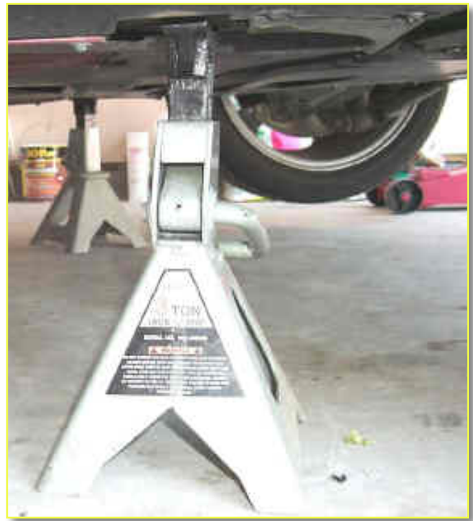
This picture shows the rear of the car resting on the jack stands
