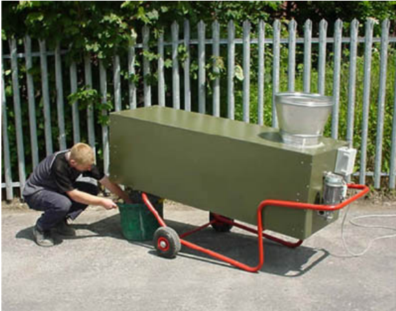
Rocket automatic continuous in-vessel composting: image www.johnstownrecycling.com
