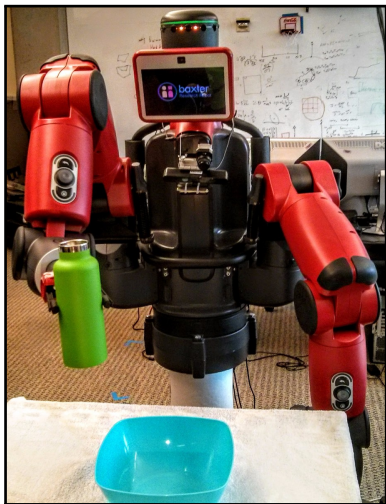
Figure 4. The robot used in the experiments in this paper. It is shown here in front of a table, holding the bottle in its right gripper, with the fruit bowl placed on the table.
