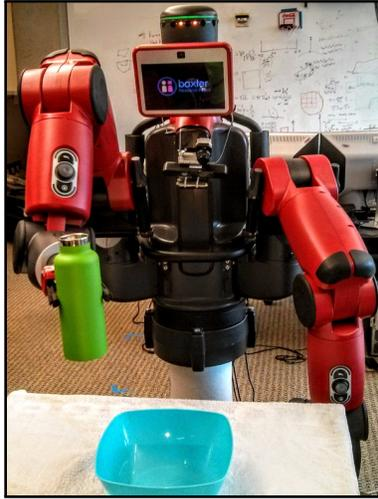
Figure 4.4: The robot used in the experiments in this chapter. It is shown here in front of a table, holding the *bottle* in its right gripper, with the *fruit bowl* placed on the table.
