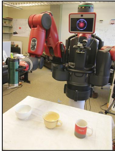
Figure 5.1: The Baxter robot used in our experiments. In its right gripper it holds the cup used as the source container. On the table in front of the robot are the three target containers (from left to right): the small bowl, tan mug, and redgray mug.
