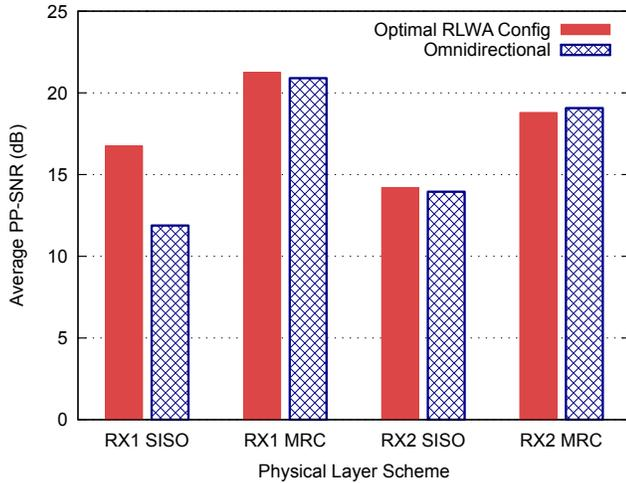
Fig. 2. The PP-SNR for Receivers 1 and 2.
