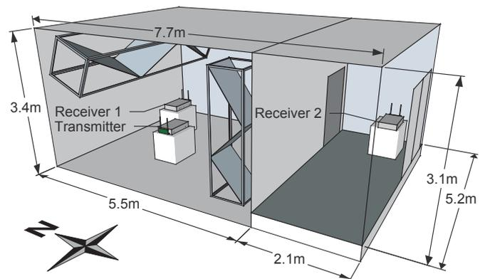
Fig. 1. Diagram of the test environment in the reverberation chamber.
