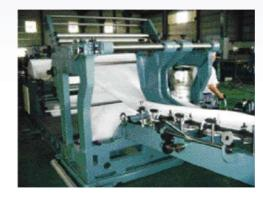
The RGT-M1 was created to tube laminated or coated flat woven fabric in facilitate client's application on rear end process of bag-making.
