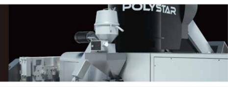
**Filter re-positioning**The re-positioning of filtration before degassing ensures a superior degassing effect, producing excellent quality pellets from heavily printed material.
