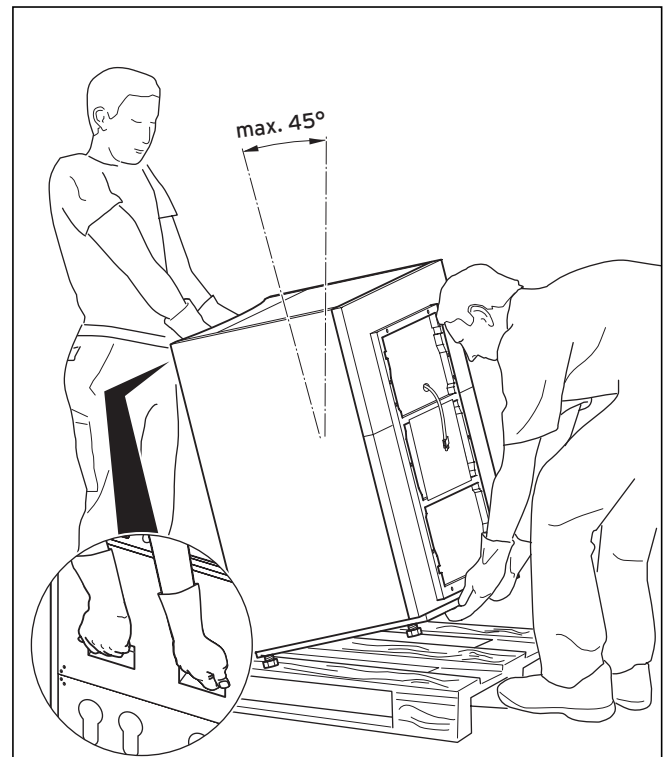
Fig. 4.6 Transporting the heat pump (carrying)
