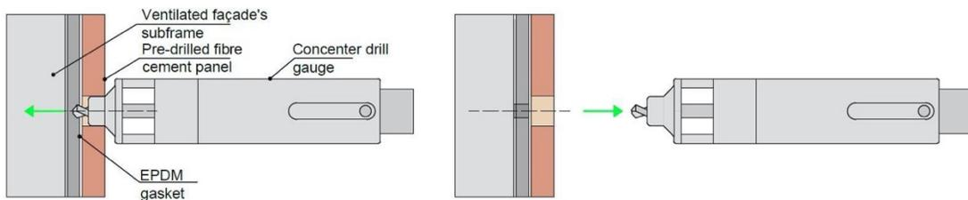
**FIXING: FIXED POINT USING THE RIVET SLEEVE AND THE RIVET**
