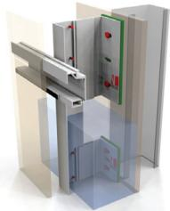
**NV5** is only suitable for Trespa Meteon HPL panels. It is a concealed fix system. Panels are supported at the bottom by the horizontal NV5 channel profile which provides restraint to panel tops.
