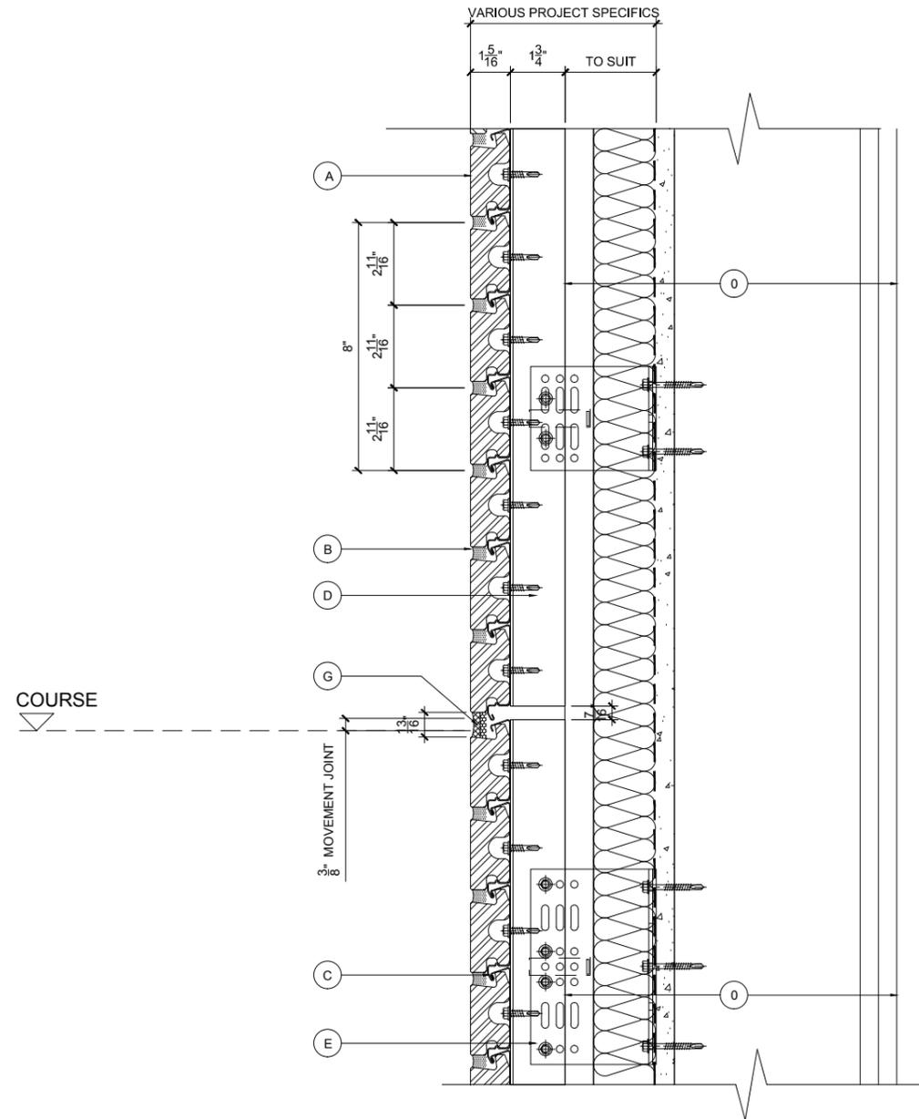
HORIZONTAL MOVEMENT JOINT DETAIL
