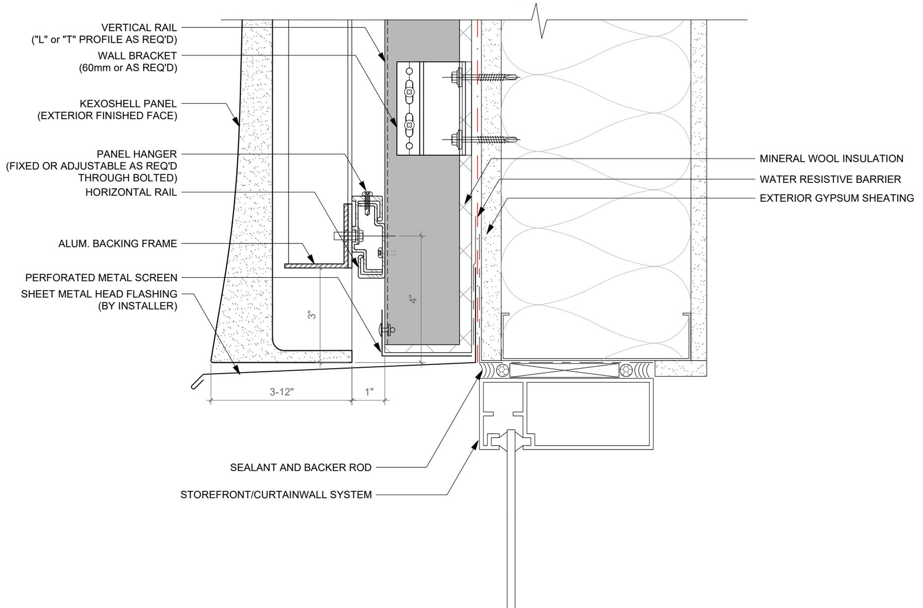
01 WINDOW HEAD DETAIL TYP. FOR PANELS WITH 3-12" D
