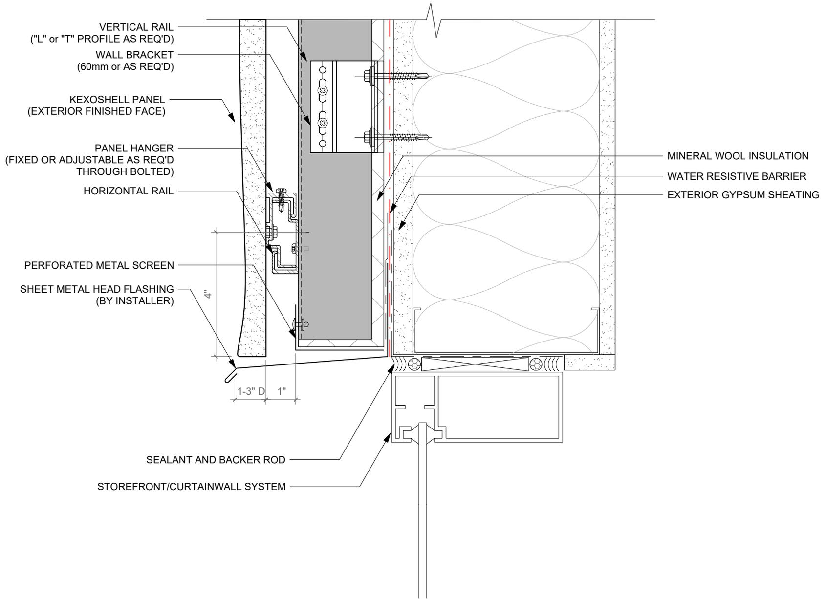
01 WINDOW HEAD DETAIL TYP. FOR PANELS WITH 1-3" D
