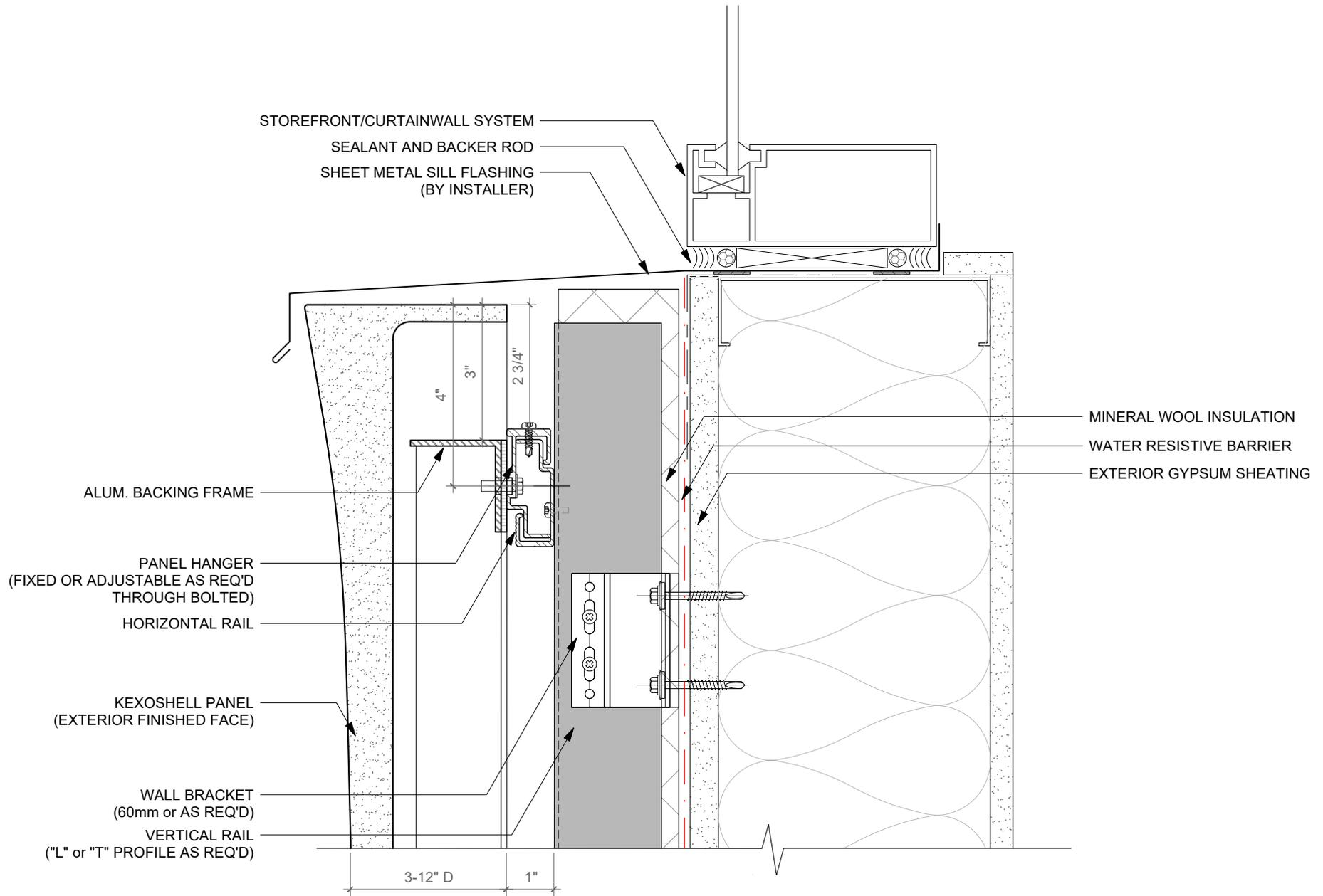
01 WINDOW SILL DETAIL TYP. FOR PANELS WITH 3-12" D
