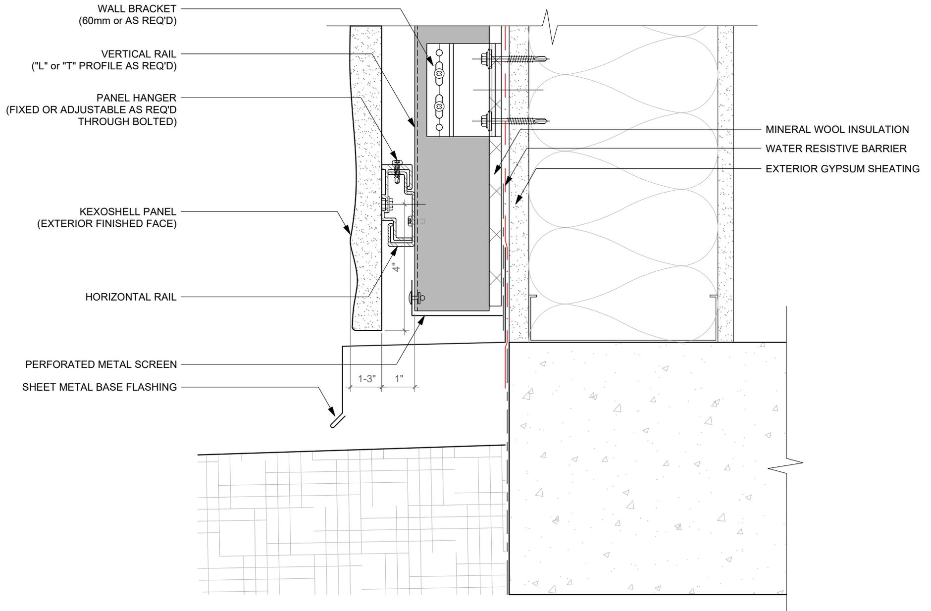
01 SECTION @ BASE DETAIL - FOR PANELS WITH 1-3" D
