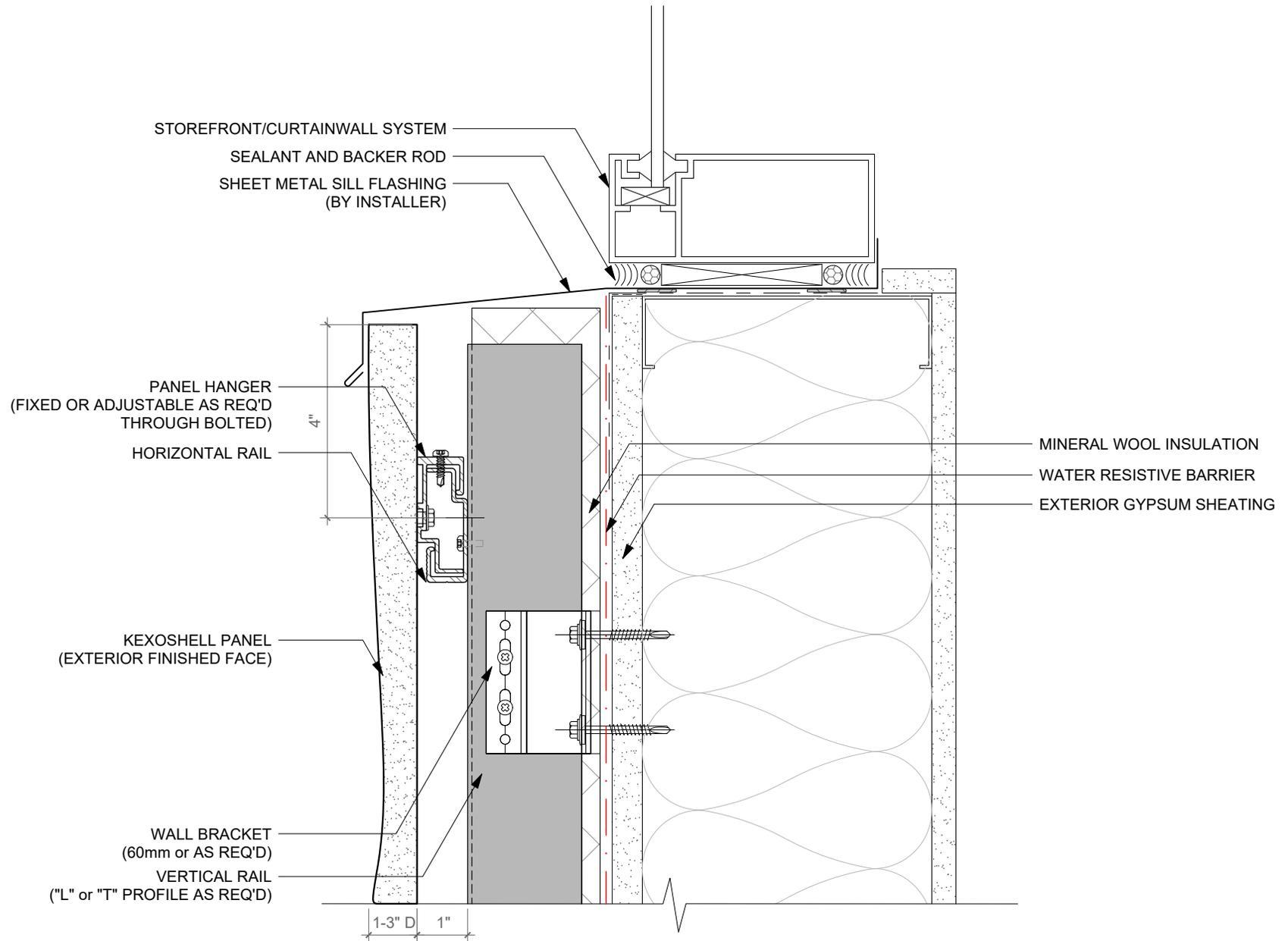
01 WINDOW SILL DETAIL TYP. FOR PANELS WITH 1-3" D
