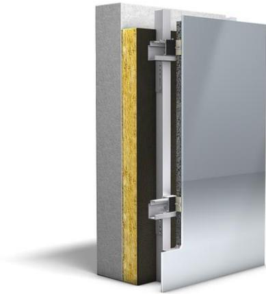
Airtec Glass is made up of robust composite panels, which can be up to 27 millimeters thick, consisting of heat-soaked thermally toughened safety glass (ESG-H) bonded to a lightweight concrete base. The panels, up to 7.74 m<sup>2</sup> in size, are hooked onto the substructure with concealed clip-type fixings. The panes of toughened safety glass are available in numerous attractive colors and can even carry customized digital printing.
