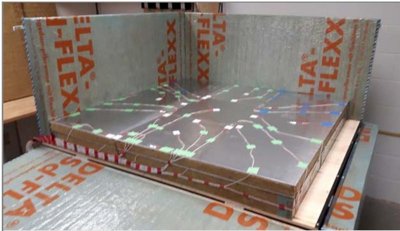
Figure 22 - Meter plate and guards.
