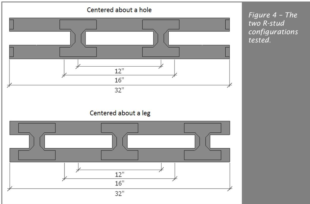
Figure 4 - The two R-stud configurations tested.
