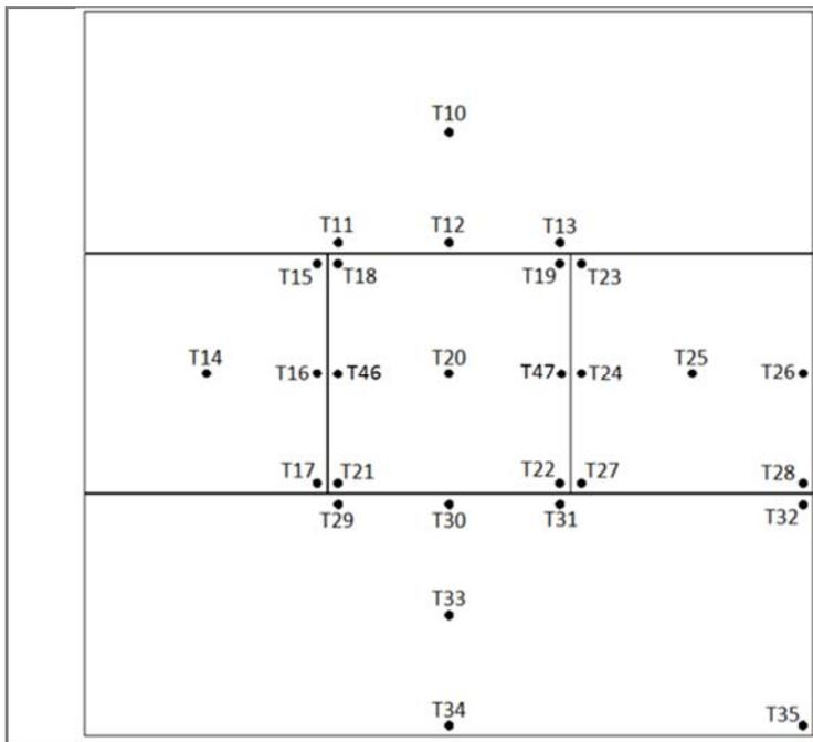
Figure 27 – Thermistor layout on the meter plate and side guards.
