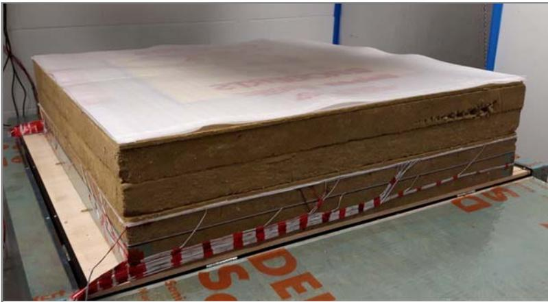
Figure 14 – Two polyethylene foam layers (representing an exterior surface film).
