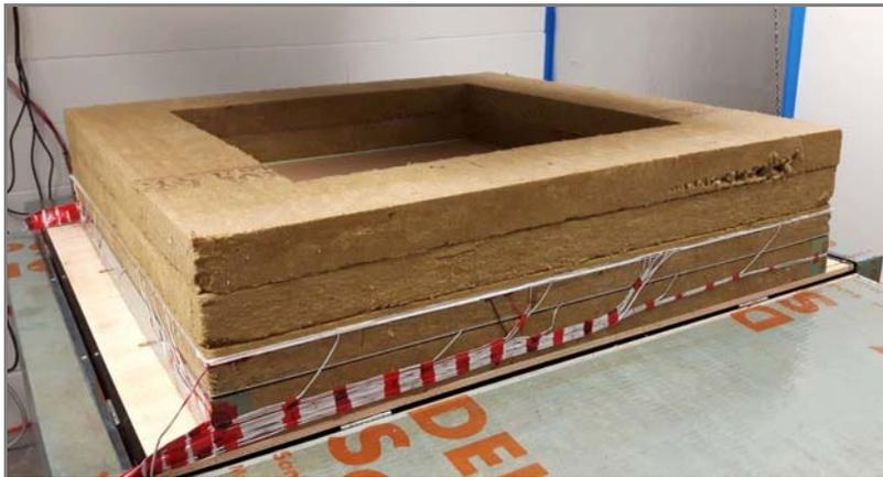
Figure 7 - The mineral wool guard around the insulation and stud layer.
