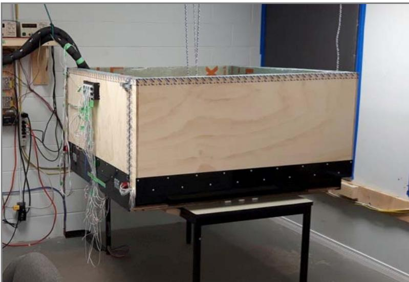
Figure 16 – Apparatus with the edge insulation panels closed around the specimen stack, ready for testing.
