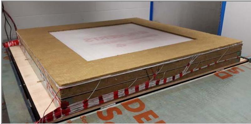
Figure 6 -The bottom mineral wool guard for around the interior gypsum board layer.
