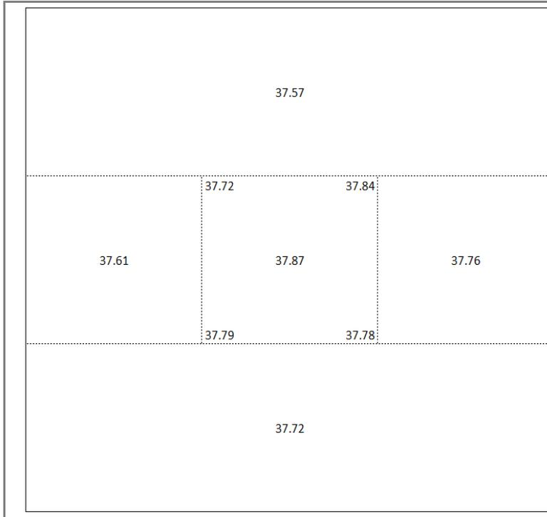
Figure 31 – Example temperature distribution (°C) on the back guard.
