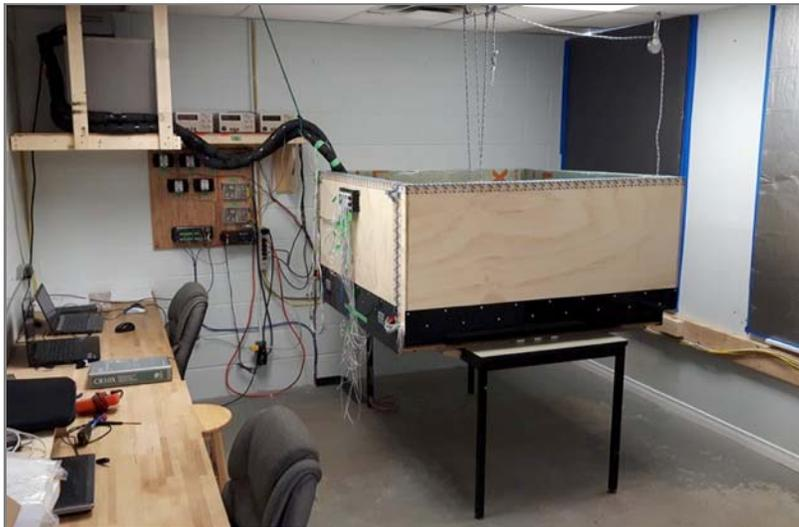
Figure 25 – Apparatus with the perimeter insulation panels closed and ready for testing.
