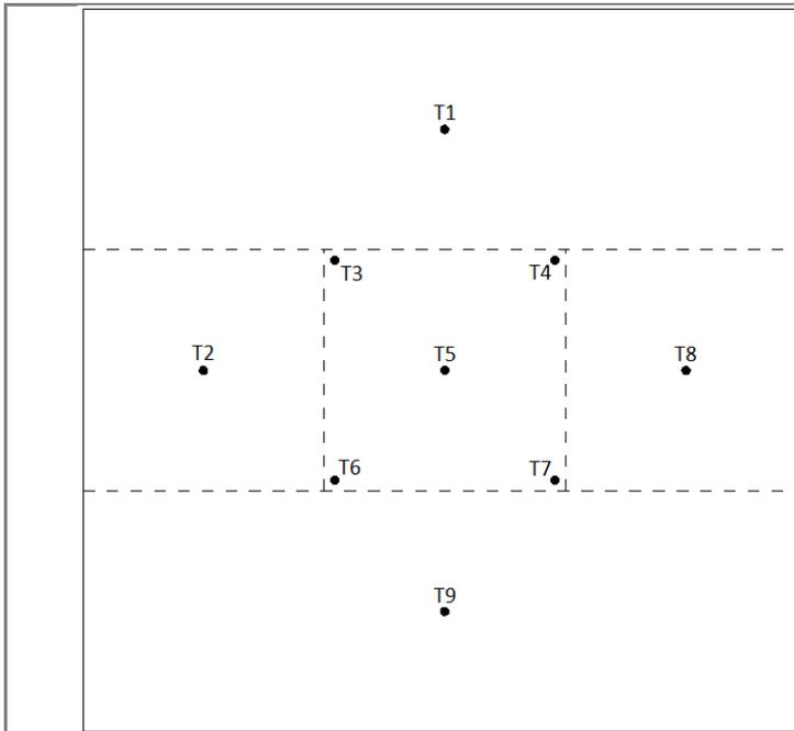
Figure 26 – Thermistor layout on the back guard.
