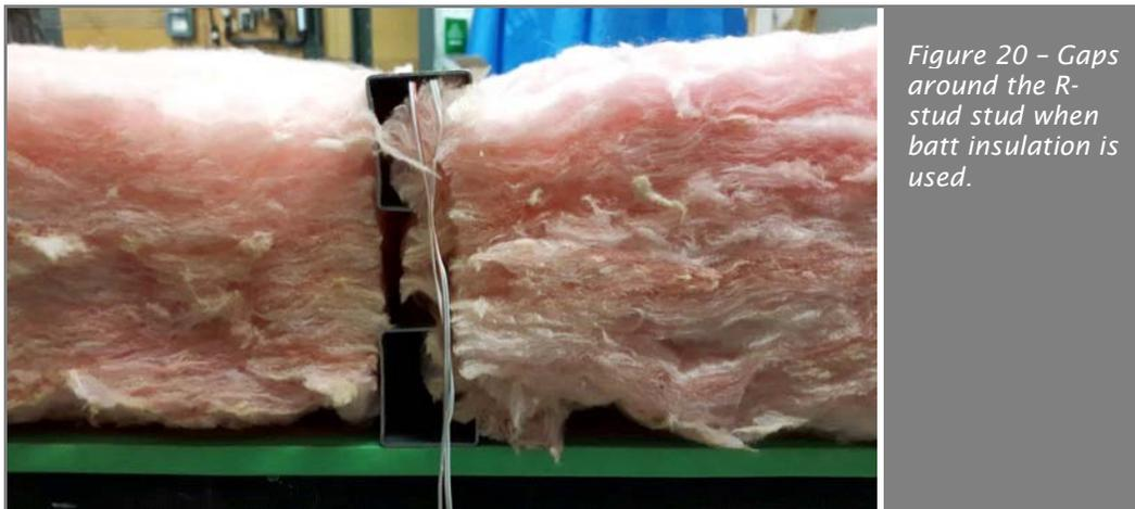
*Figure 20 - Gaps around the R-stud stud when batt insulation is used.*
