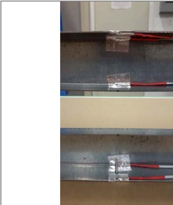
*Figure 19 - Close-up view of the additional sensors at the middle of the track.*
