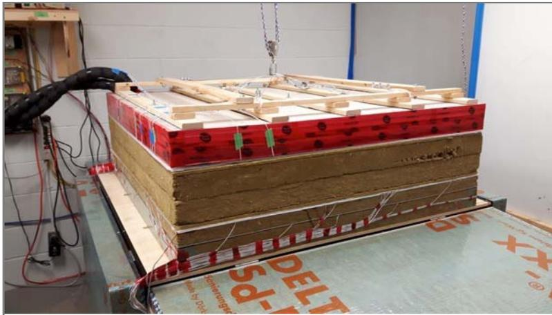
Figure 24 - Apparatus with the perimeter insulation panels open.
