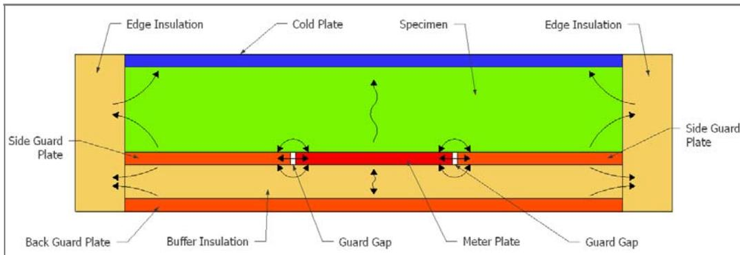
*Figure 21 – Cross-section schematic of the guarded hot plate apparatus.*
