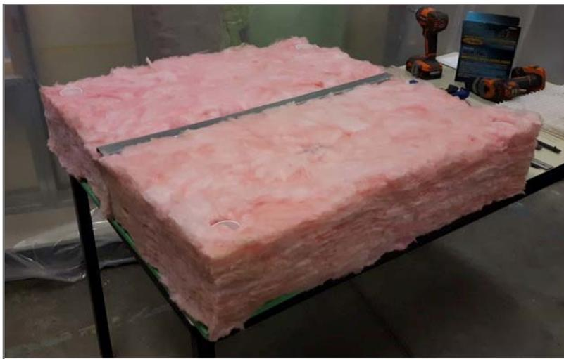
Figure 9 - Fiberglass batt insulation installed around the standard stud. Thin PVC pipe spacers are placed at the corners outside of the meter area to ensure the 6" stud cavity is maintained.
