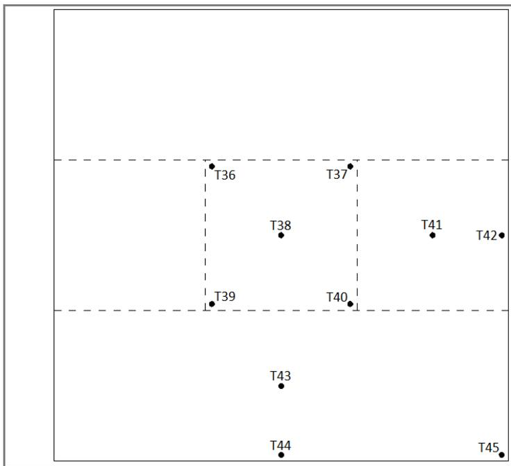
Figure 28 – Thermistor layout on the cold plate.
