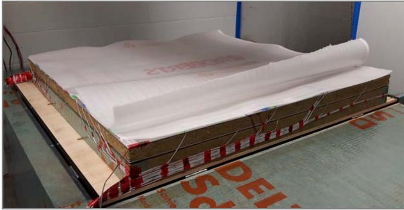
Figure 5 - The bottom two layers of polyethylene foam (representing an interior surface film).
