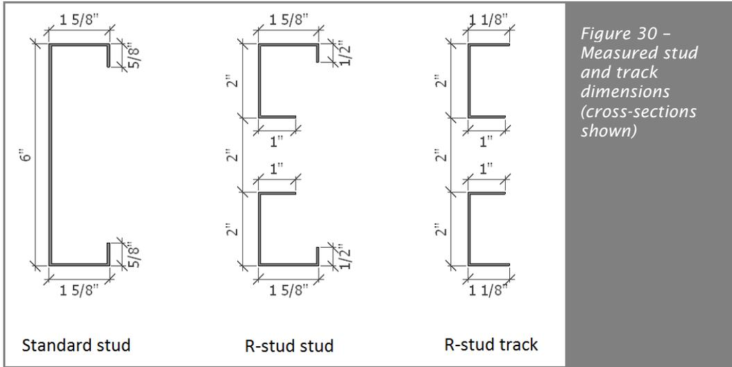
Figure 30 – Measured stud and track dimensions (cross-sections shown)
