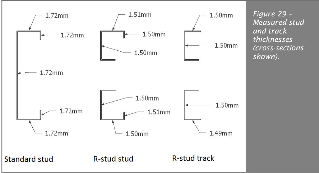
Figure 29 – Measured stud and track thicknesses (cross-sections shown).
