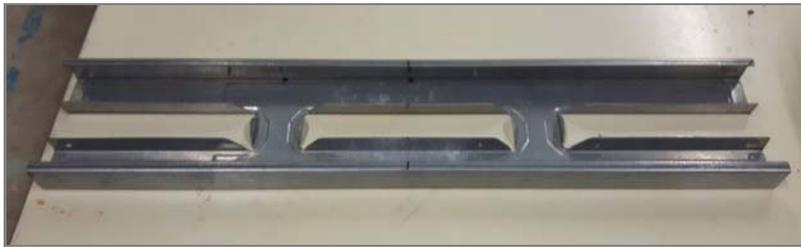
*Figure 2 – One of the R-stud studs used in the assemblies.*
