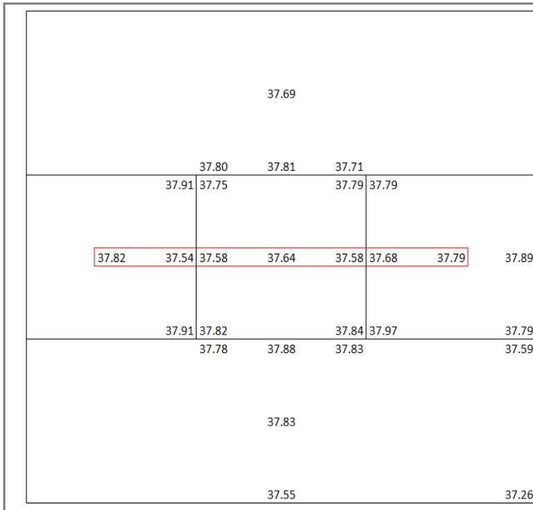
Figure 32 – Temperature distribution (°C) on the meter plate and side guards. Stud location outlined in red.
