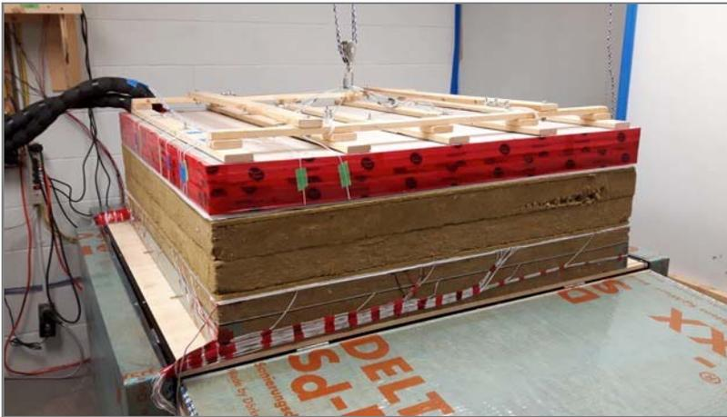
Figure 15 – Cold plate installed on top of specimen stack. The edge insulation panels fold up to guard the entire stack from ambient conditions.
