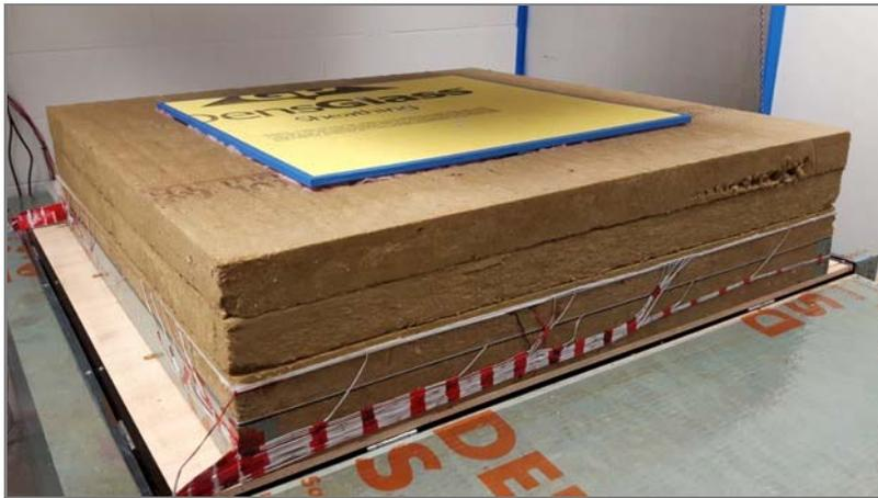
Figure 11 - Wall assembly installed surrounded by mineral wool guard.
