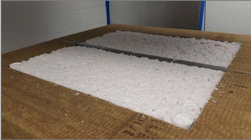
*Figure 17 -Blown fiberglass installed within the R-stud assembly.*
