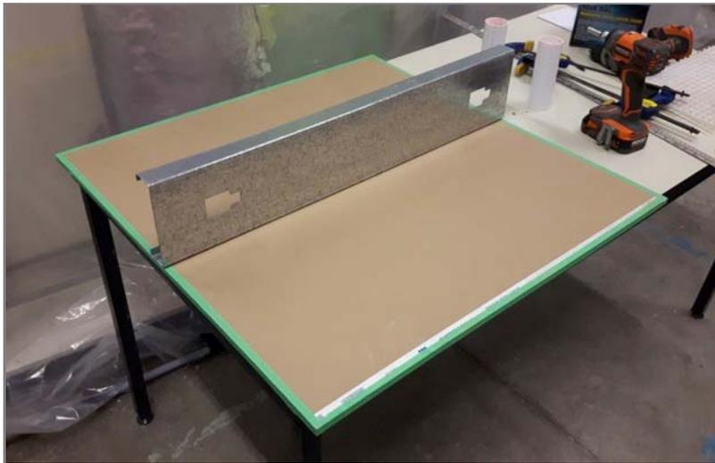
Figure 8 -Steel stud screwed to the interior gypsum board.
