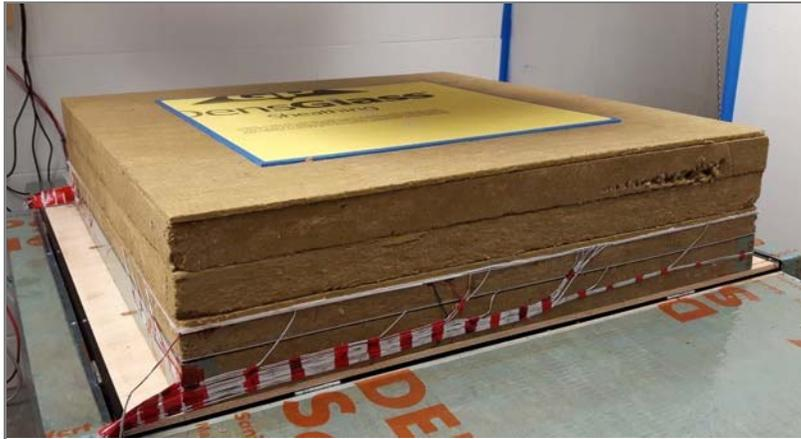
Figure 12 - Top mineral wool guard piece around the exterior gypsum wallboard.
