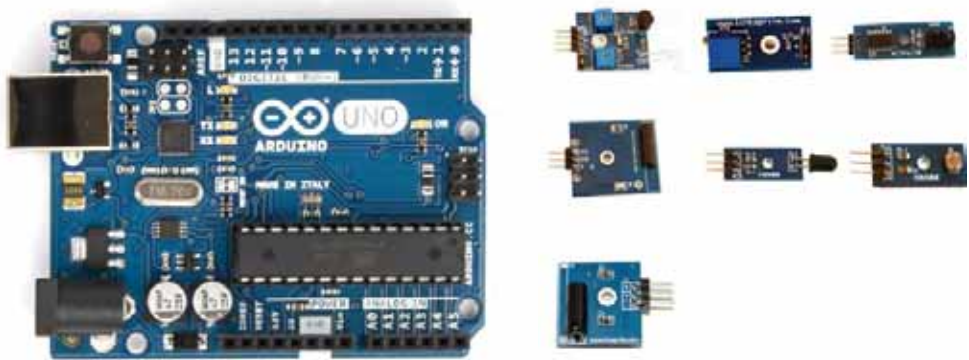
Figure 1: Arduino Uno Microprocessor with Sensors Kit. Source: Arduino.com
