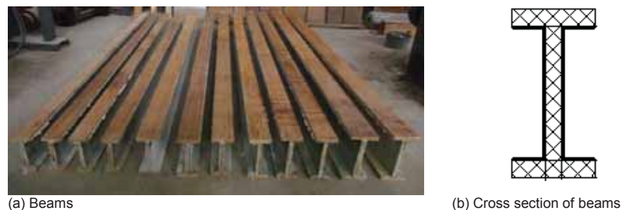
Figure 5: Bamboo-steel composite beam.
