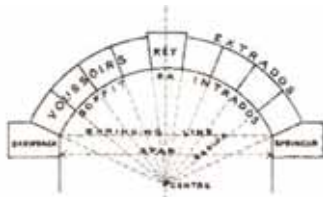
Figure 2: Segmented arch with defined terms: (Purchase 1904)
