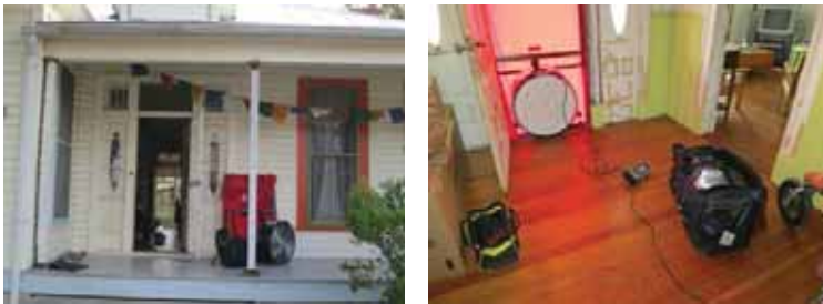
Figure 2: Door blower testing performed for case study homes.
