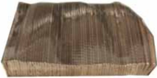
Figure 2: Plexi Vacuum formed on cardboard (Smith 2014)
