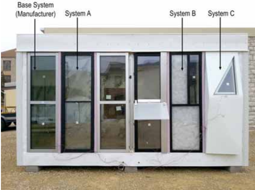
Figure 1: Image showing test structure and 1:1 scale prototypes constructed by the students for thermal testing. Source: (Author 2014)
