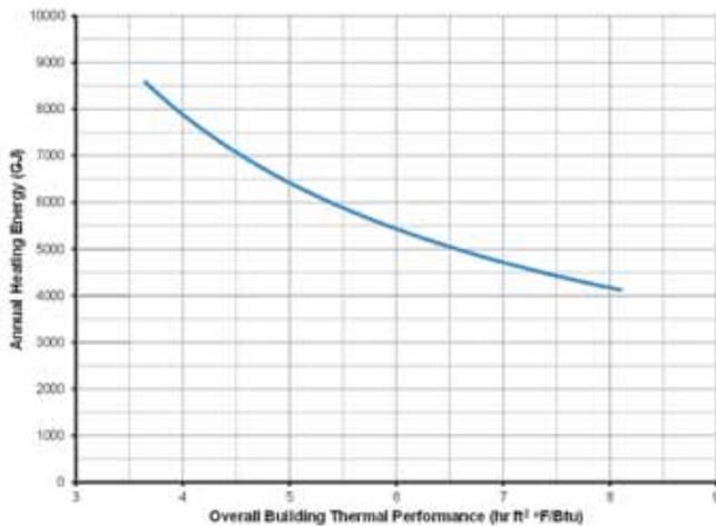
Figure 7. Energy use versus overall building thermal performance for the study building.
