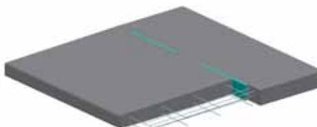
b. Site solution with intermittent reinforced concrete and rigid insulation
