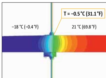
Conventional solution (continuous concrete slab)
