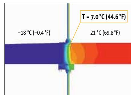
MSTB providing significantly improved interior surface temperatures
