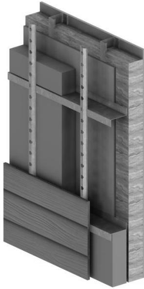
**Figure 5:** Vapour Resistances of Example Steel Stud Wall Assembly with Split Insulation
