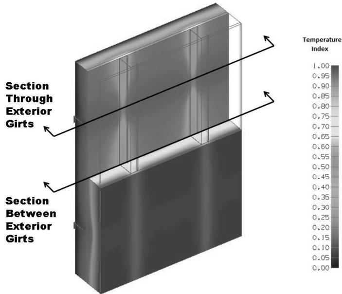
**Figure 2:** Temperature Distribution of a Steel Stud Assembly with 3D Heat Flow Paths
