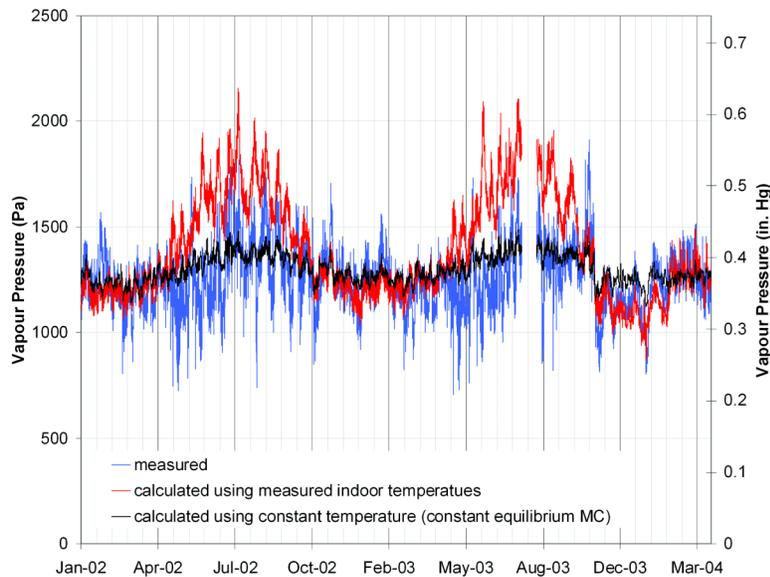
**Figure 7** Comparison of measured and calculated indoor vapour pressure for different indoor temperatures.
