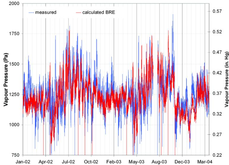
**Figure 8** Comparison of measured and calculated indoor vapour pressure for changes parameters for different seasons.
