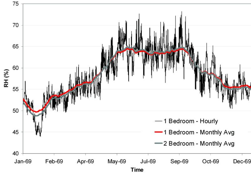
Figure 10 Monthly average indoor RH calculated with BRE Admittance Model and parameters in Table 5.
