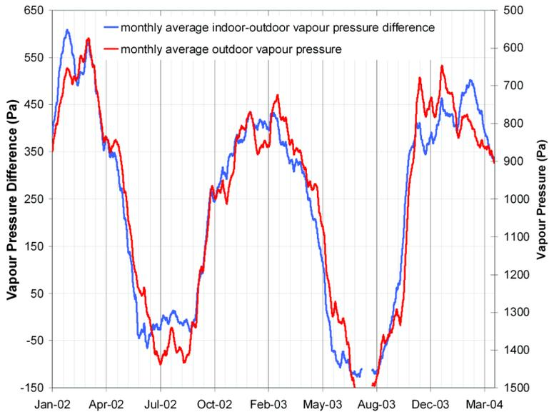
**Figure 5** Comparison of measured indoor-outdoor vapour pressure difference to outdoor vapour pressure.
