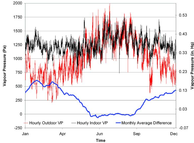
**Figure 4** Comparison of measured indoor vapour pressure and outdoor vapour pressure.
