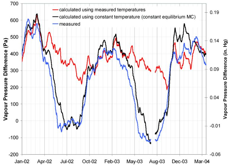
**Figure 6** Comparison of measured and calculated indoor-outdoor vapour pressure difference for different indoor
