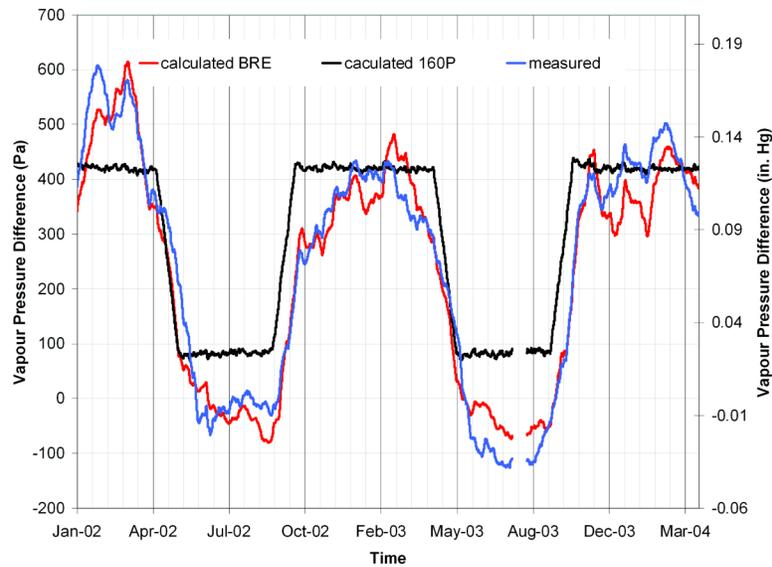
Figure 9 Comparison of measured and calculated indoor vapour pressure.
