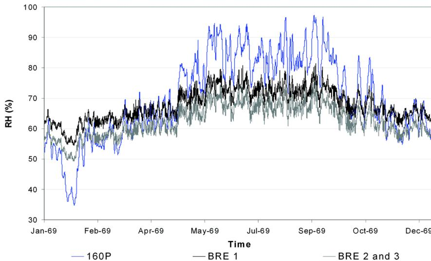
**Figure 2** Comparison of relative humidity calculated using ASHRAE 160P and BRE approaches with moisture generation rates as recommended by ASHRAE 160P and with Vancouver (1969) climatic data.
