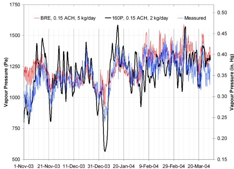
**Figure 1** Comparison of the 160P and BRE approaches to measured data of a multiunit residential building during the heating season for a mild marine climate (Vancouver).
