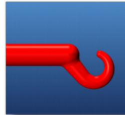
Optimum gate geometry, with edges rounded
