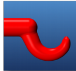
Optimum gate geometry, with edges rounded
