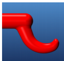
Optimum gate geometry, with edges rounded
