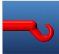
Optimum gate geometry, with edges rounded
